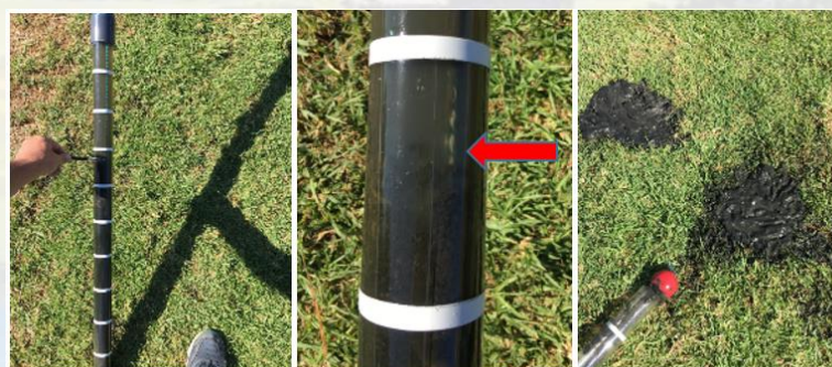
Sample 2: 780mm / 110mm compacted sludge
